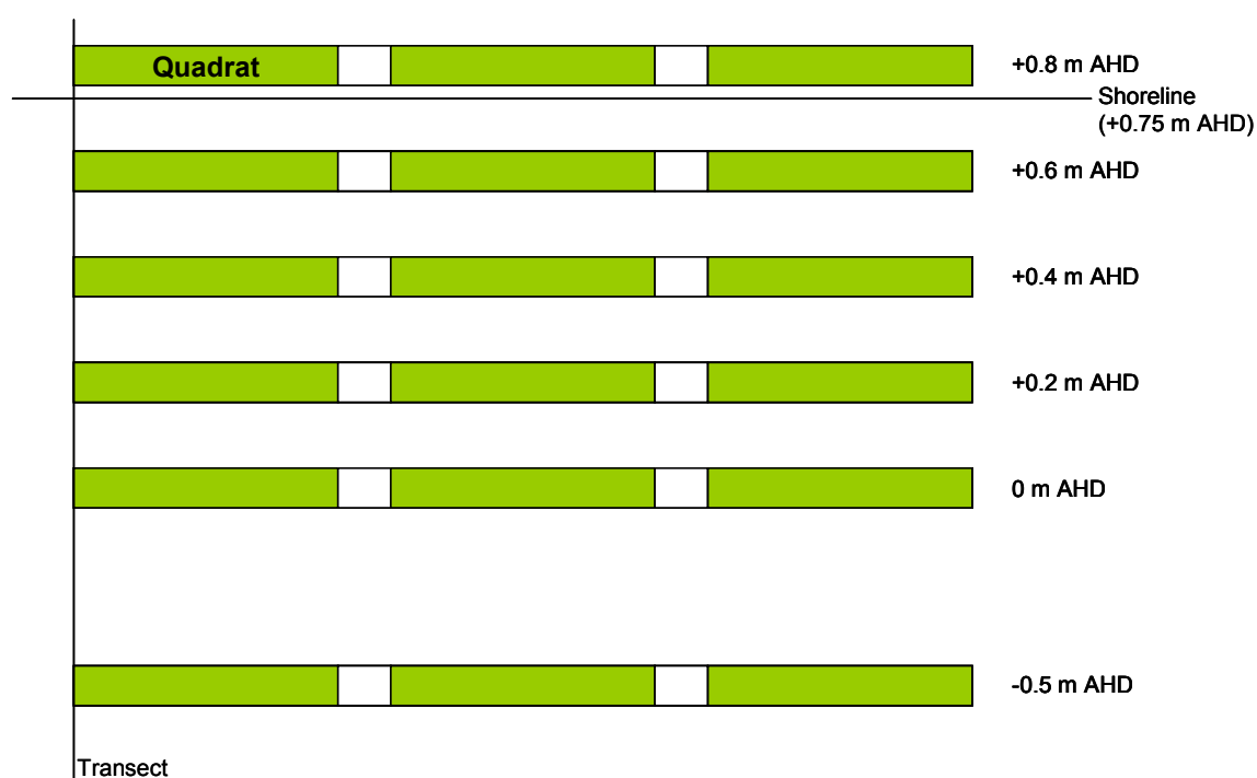
Figure 4: Vegetation surveying protocol for lakeshore sites: plan view showing placement of quadrats relative to the shoreline.
